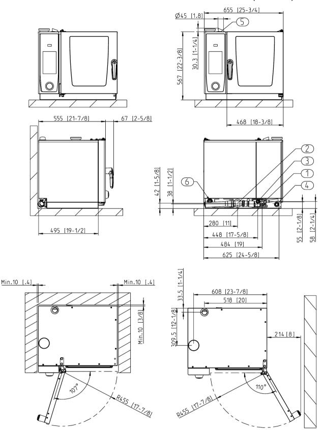
1. Common water supply (cold water) "Single" water connection as shipped 2. Drain 3. Electrical connection wire entrance 4. Chassis Ground connection 5. Steam Vent pipe 2 3/8" / 60mm Minimum Clearance 2" / 50 mm Left side clearance 20" recommended for servicing of unit without the ability to move unit while connected. Measurements in mm (inch)
